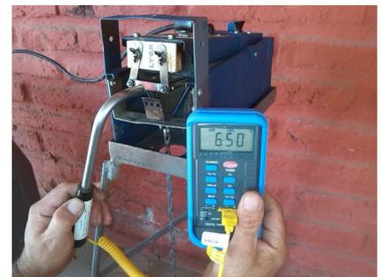
Pyrometer indicating proper blade temperature of 650°C.
